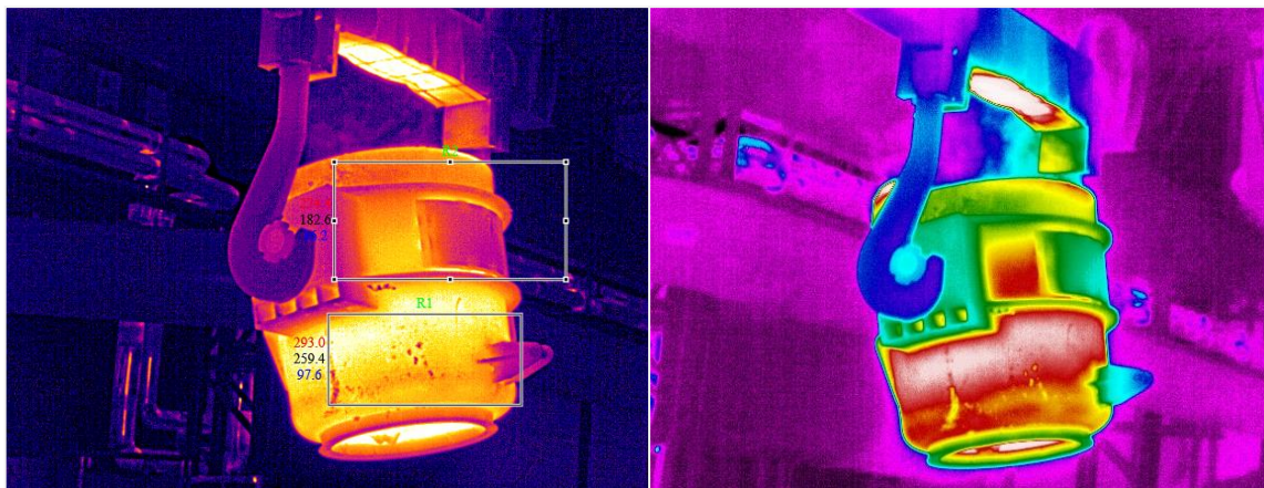
Figure 6.1 Defect Monitoring of Ladle Resistant Material
