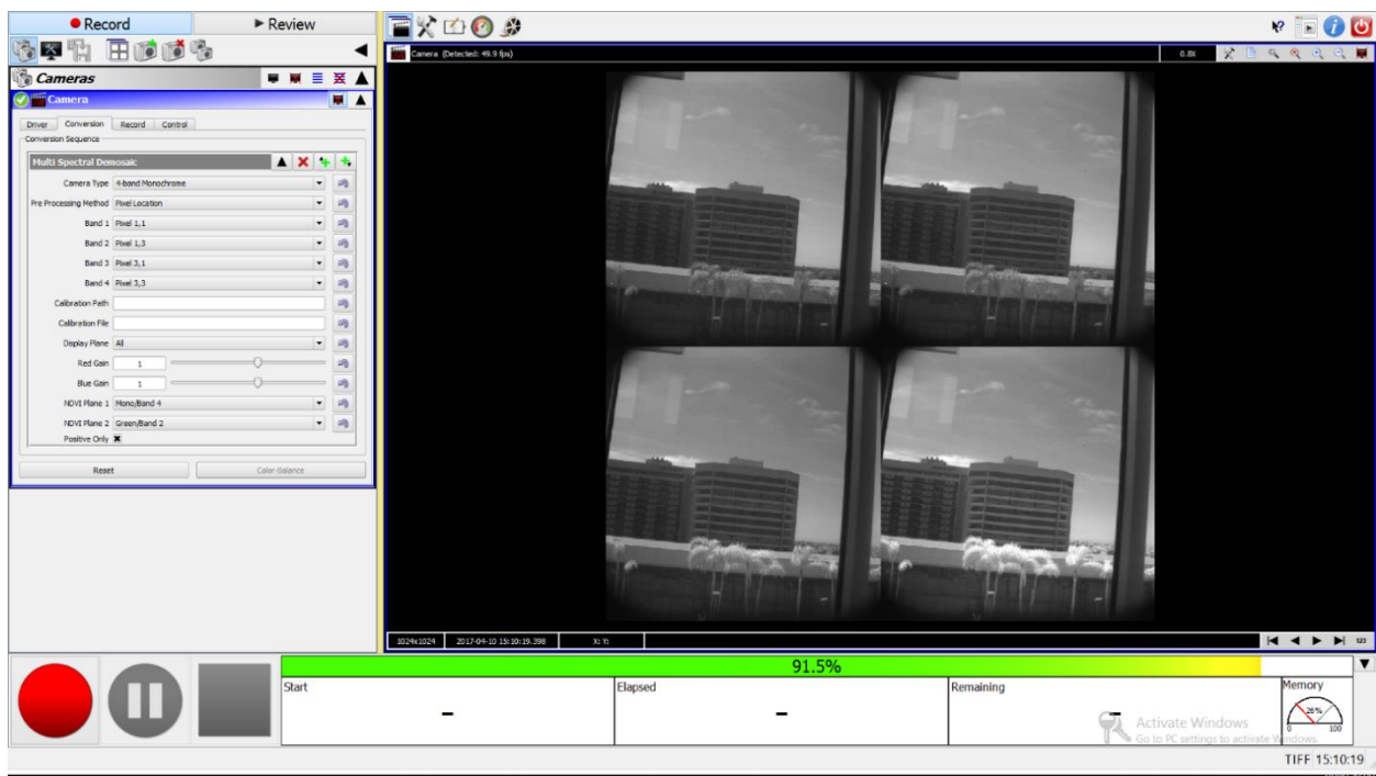
Figure 10.3. Real-time display of multispectral images in montage format. Example here collected with 4-band multispectral camera for agriculture.
