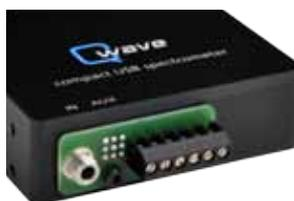
The Qmini includes 4 I/O channels that can be configured as trigger input, shutter and light source control or general purpose I/O pins. The optional I/O adapter provides easy access via a screw terminal block.
